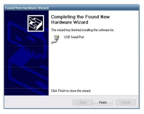
The RS-485 cable behaves as virtual com port (VCP). A number is assigned to the VCP in the Control panel/System/Device Manager under Ports (COM & LPT). This port number is used to set the communication parameters in the **Set communication properties** window of the BMS Control software.
